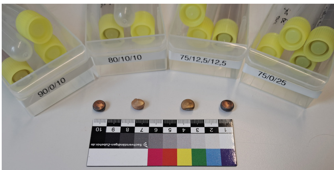
Figure 5: Four produced reference samples of lead-bronze coins used in this work
